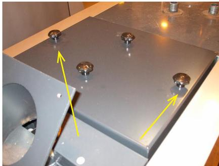
1. Open the outer star knobs and remove the cleanout hatch.
