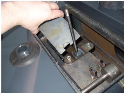
4. Lift the lift lever up, remove the hatch for the convection channel.
