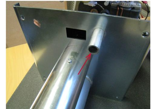
Clean the metal pipe of the flame detector so that the ash accumulated in the pipe will not hinder the operation of the flame detector.
