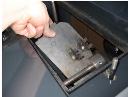
5. Lift off the second hatch of the convection channel.
