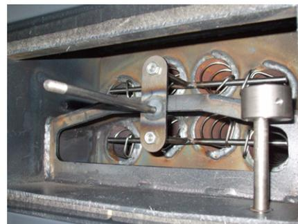
8. Reinstall all the springs and lifting levers illustrated.
