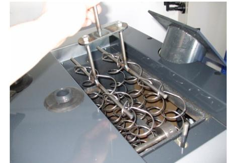
6. Lift off the holder and the springs from the convection.
