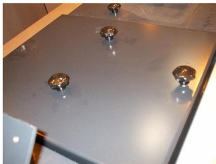
8. Attach the cleanout hatch and fit the star knobs.
