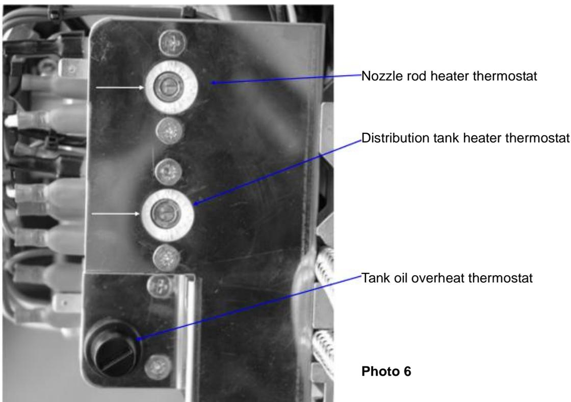
**WARNING!** Do not exceed the temperature of 90 °C. Any higher temperature poses a risk to the thermocouples and presents the hazard of the floater sensors burning away.
