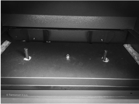
Metal cap with tubulator lifters and one screw in the middle is visible.
