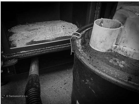
Clean the area inside with the ash cleaner or using manual tools. When screwing back the holders, screw completely, so that no air can pass inside.
