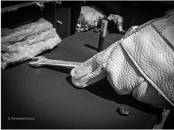
With fork-key size 13 or boiler KEY, unscrew the upper cover of the heating chamber.
