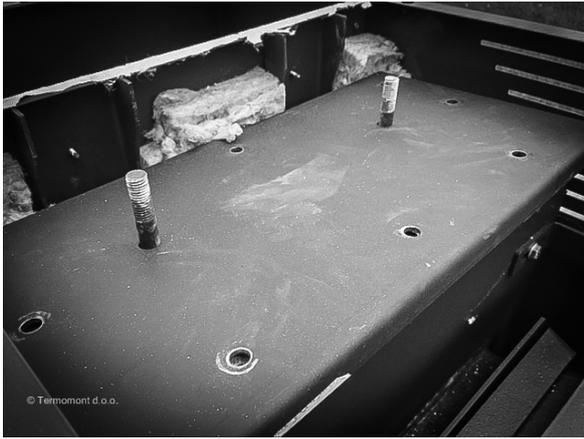
After the cleaning put back the cover and screw the holders.
