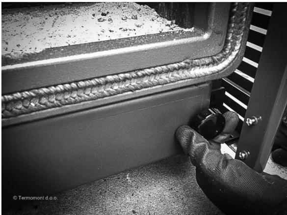
Release the screw-balls that hold the plate below.
