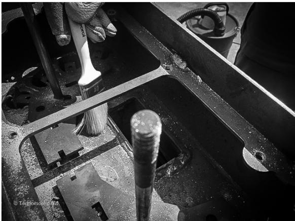
Perform detailed cleaning of all parts that can be accessed. Remove the ash.
