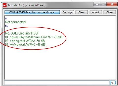
12.) Pick up the network you would like to use for WiRCU module and very carefully follow our example. Remark: Wireless networks with WEP encryption are not supported because of too low security standards.
