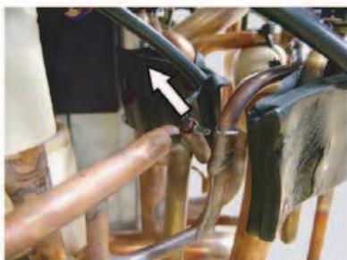
Remove the THERMISTOR SPRING.
