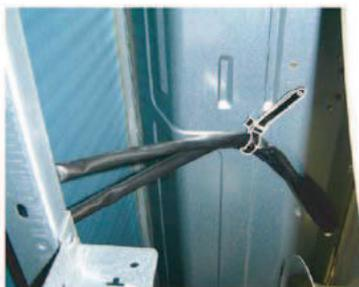
Loose the clamp, and remove the lead wires
