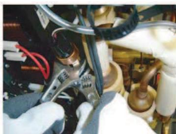
Remove the PRESSURE SENSOR with wrench.
