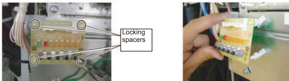
Remove the connectors and locking spacers.
