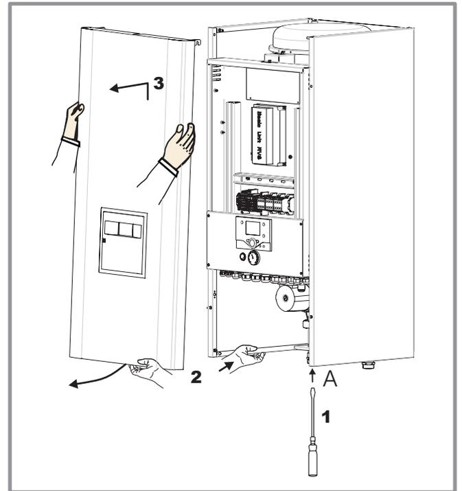
**Figure 16 - Removing the front facing**
