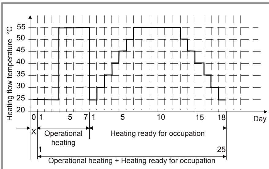
Figure 44 - Diagram of the concrete slab drying programmes
