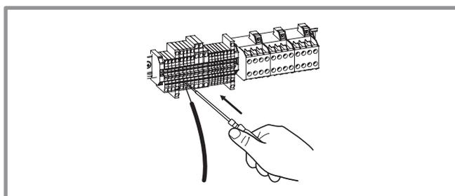
Figure 30 - Hydraulic module terminal block
