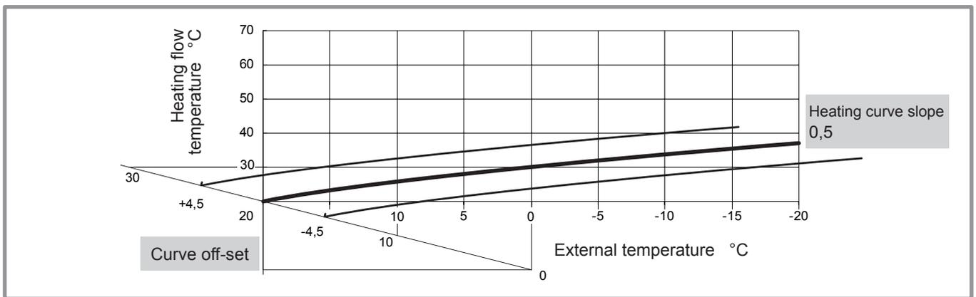
Figure 42 - Off-set of the heating curve (line 721)
