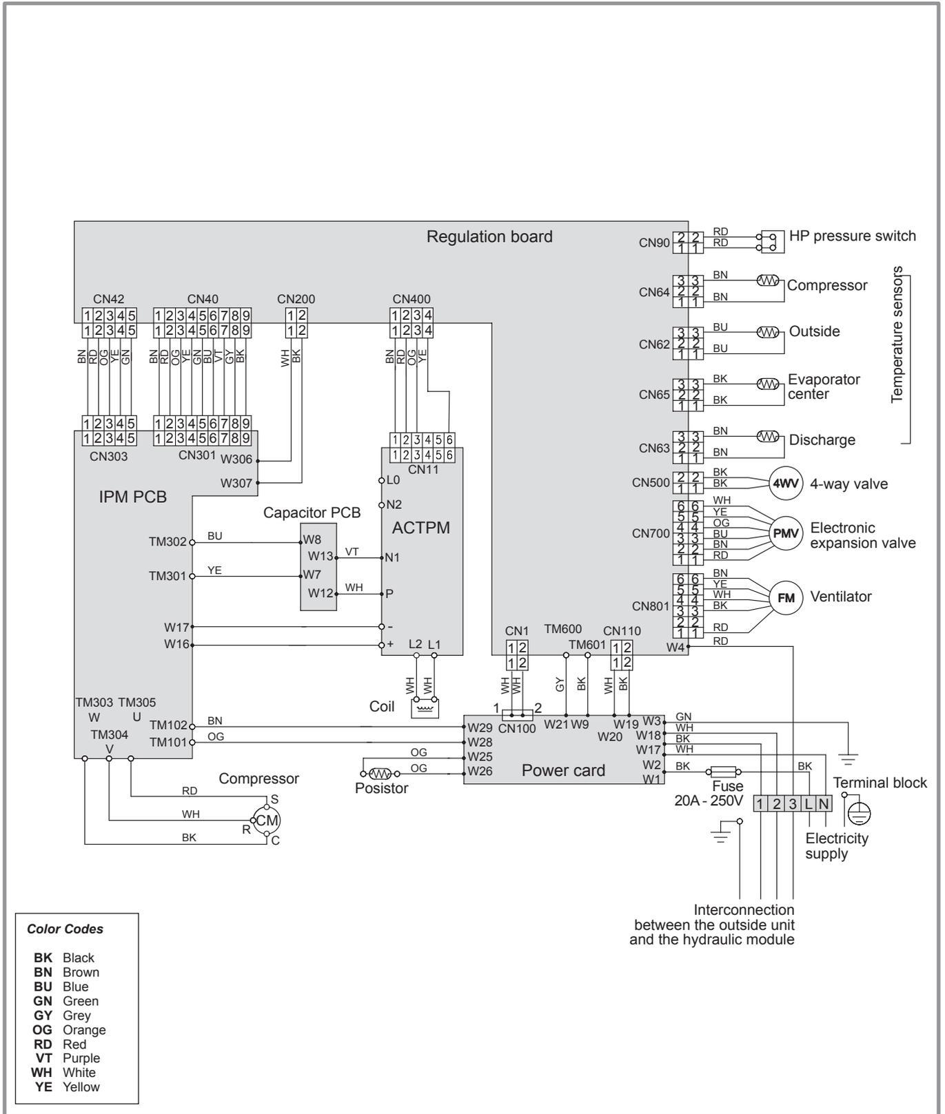
Figure 46 - Electrical wiring of outside unit (model S10)
