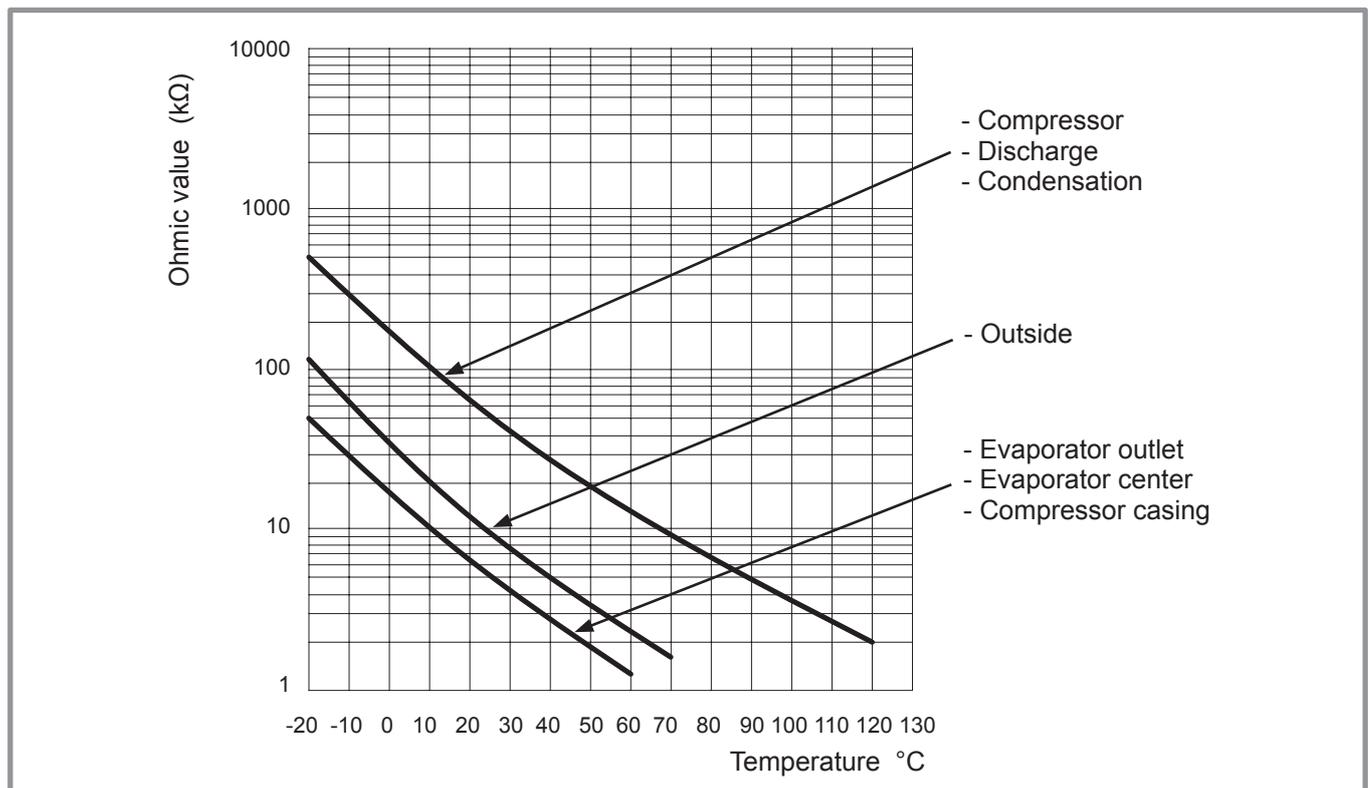
Figure 6 - Ohmic values of the sensors (outside unit)
