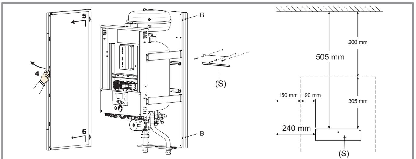
**Figure 17 - Removing the sides and fixing the support (S)**
