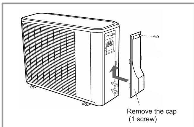
**Figure 32 - Access to outside unit's terminal block (model S5, S6, S8)**
