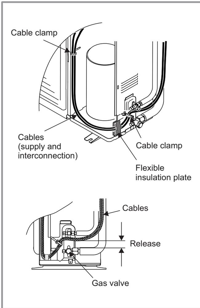
**Figure 35 - Finalisation of connection to outside unit**
