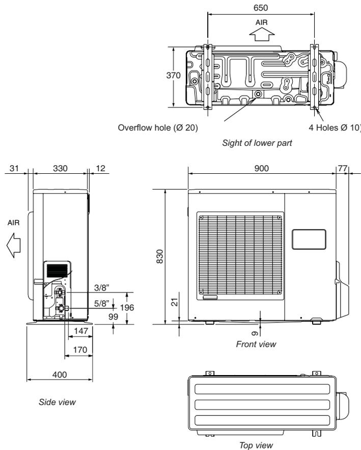
Figure 1 - Dimensions in mm
