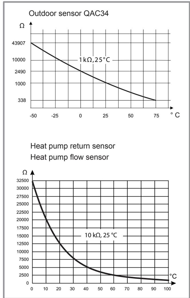
Figure 5 - Ohmic values of the sensors (Hydraulic module)
