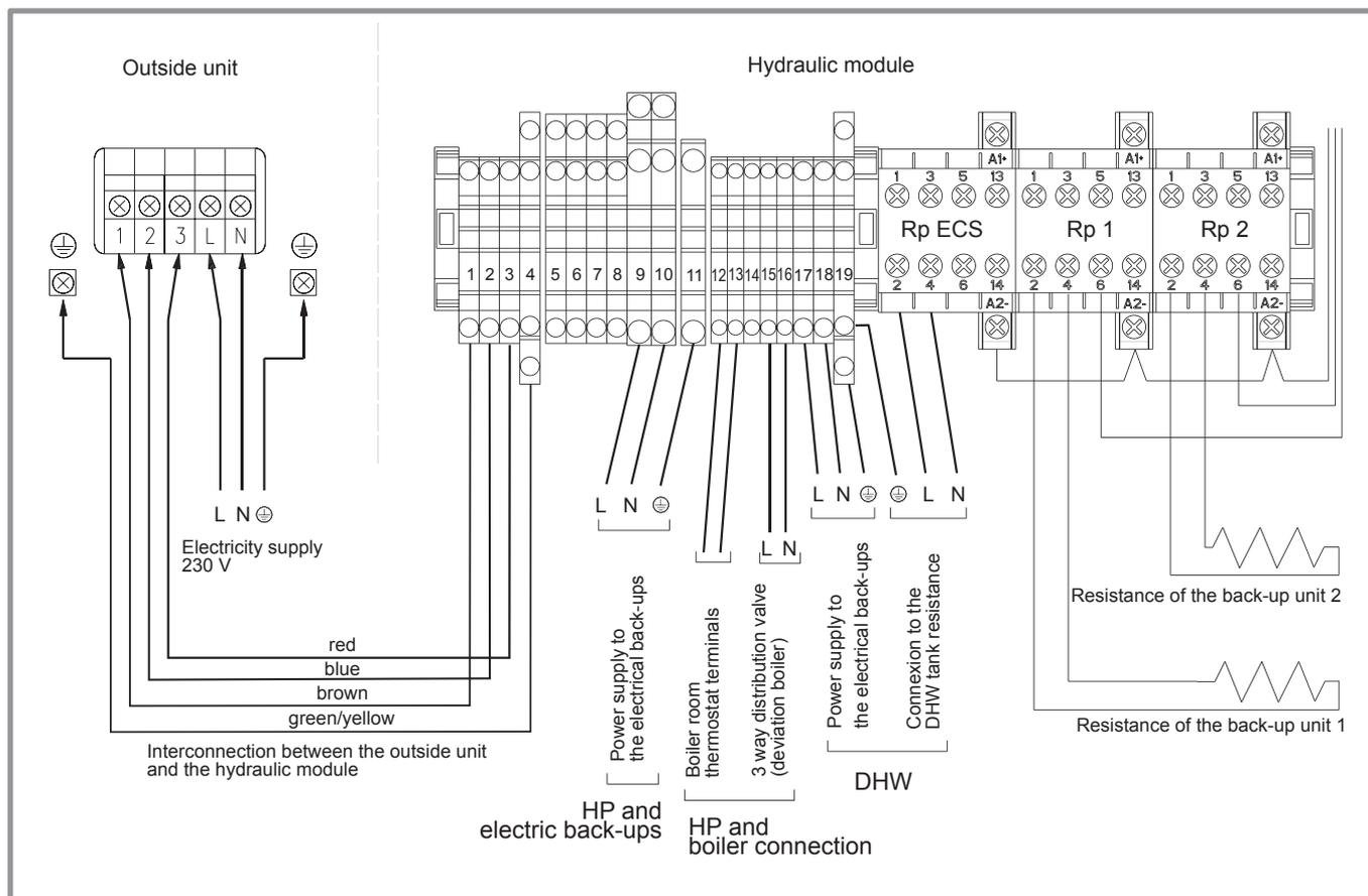
Figure 37 - Connection to terminal block and power relays
