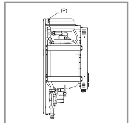
**Figure 27 - Hydraulic module bleeder valve**
