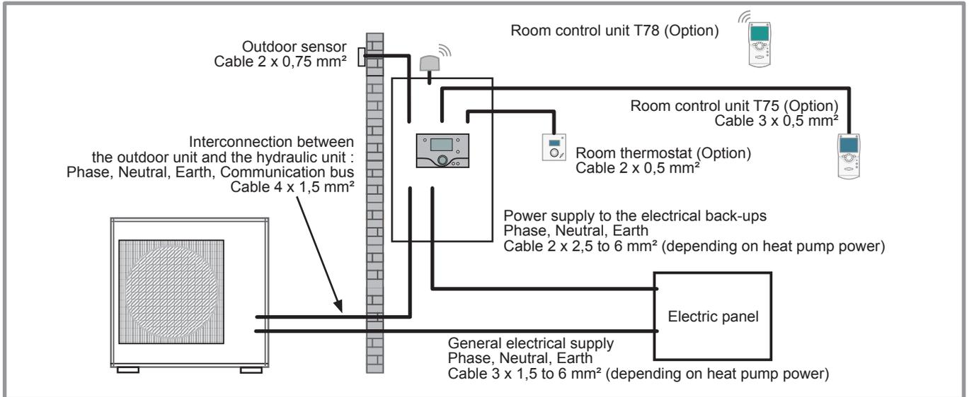
Figure 31 - Overall layout of the electrical connections for a simple installation (1 heating circuit)
