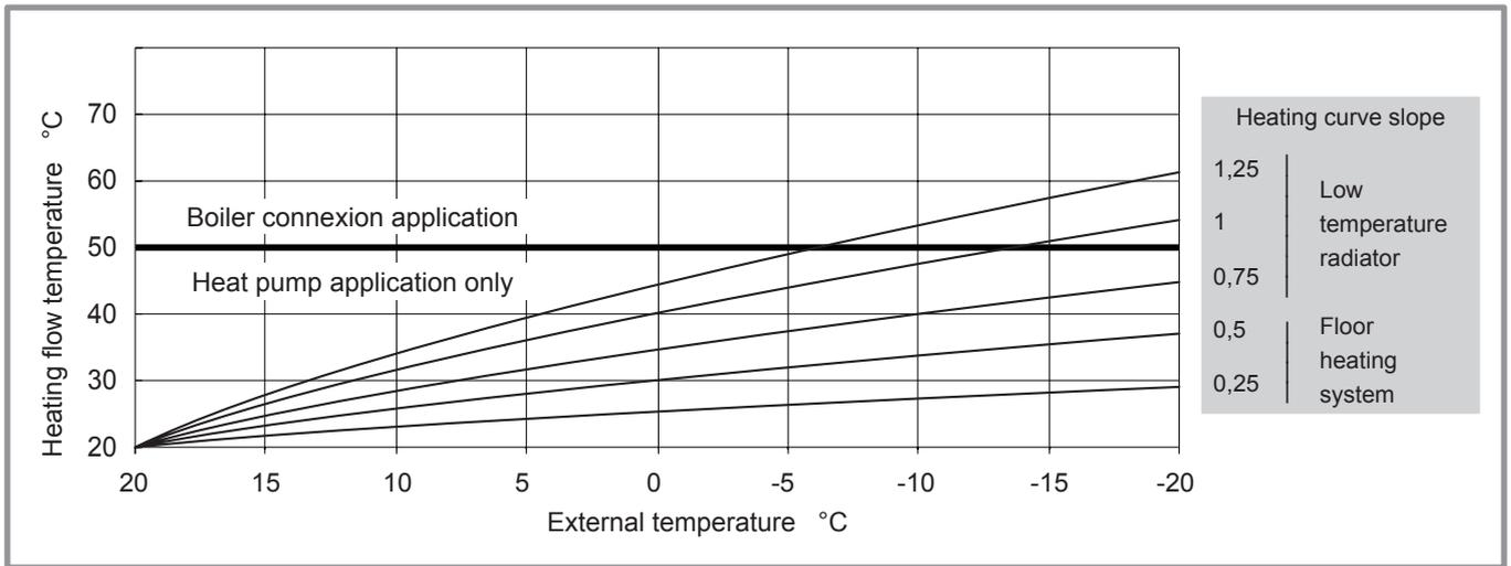
Figure 41 - Heating curve slope (line 720)
