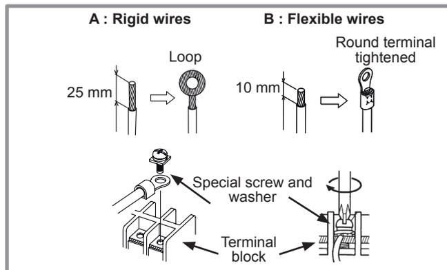
Figure 28 - Outside unit terminal block
