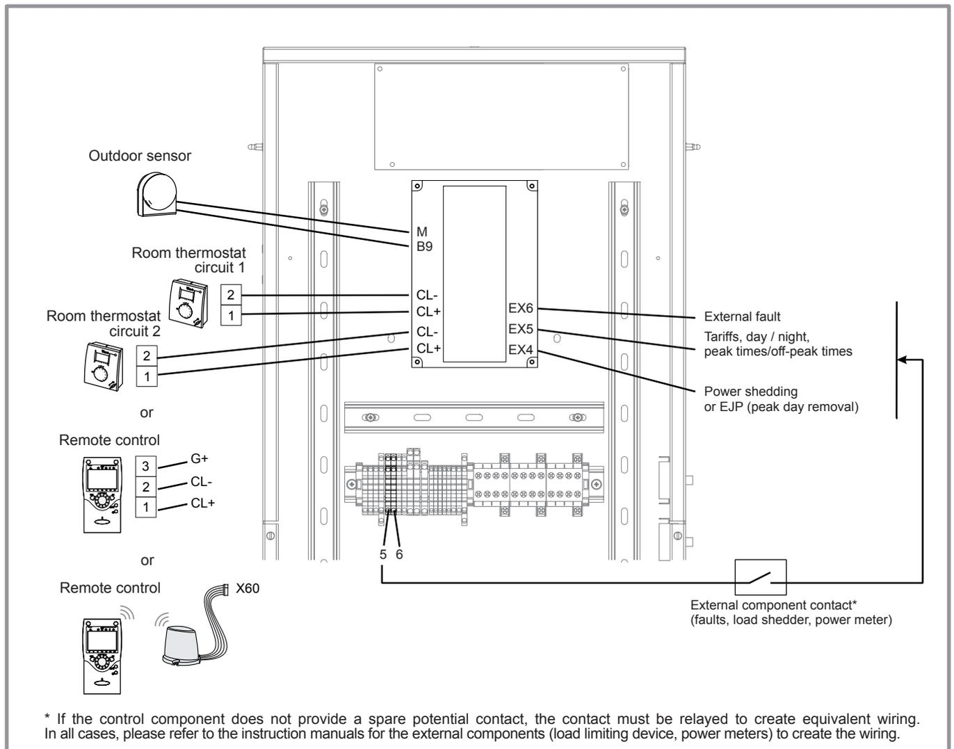
**Figure 38 - Connections to the heat pump regulator (accessories and options)**
