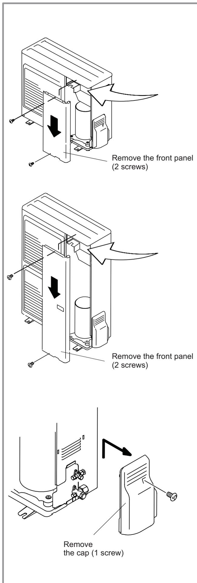
**Figure 34 - Access to outside unit's terminal block (model S10, S13, S16)**
