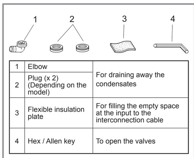
Figure 10 - Accessories provided with the outside unit
