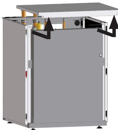
◆ **Removing the indoor unit lateral cover**
